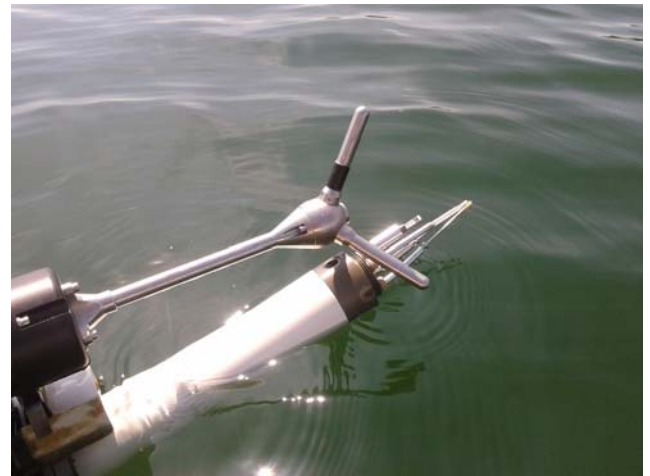
Figure 3 : Microprofiler (Scamp) coupled with ADV
