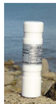
Figure 23 : water temperature and pressure sensors (nke SP2T10)
