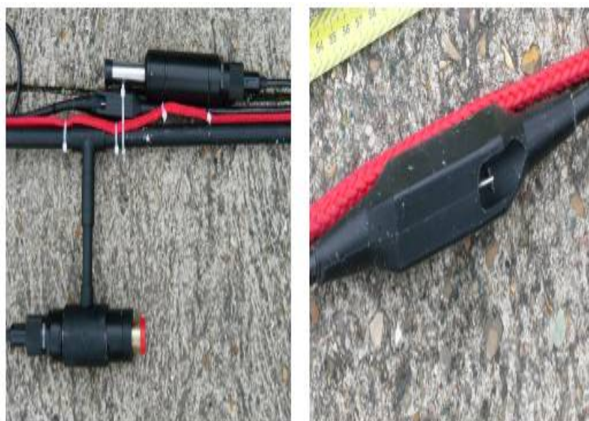
Figure 22 : Chlorophyll fluorescence, photosynthetically active radiations (PAR) sensors (on the left) and water temperature (on the right)
