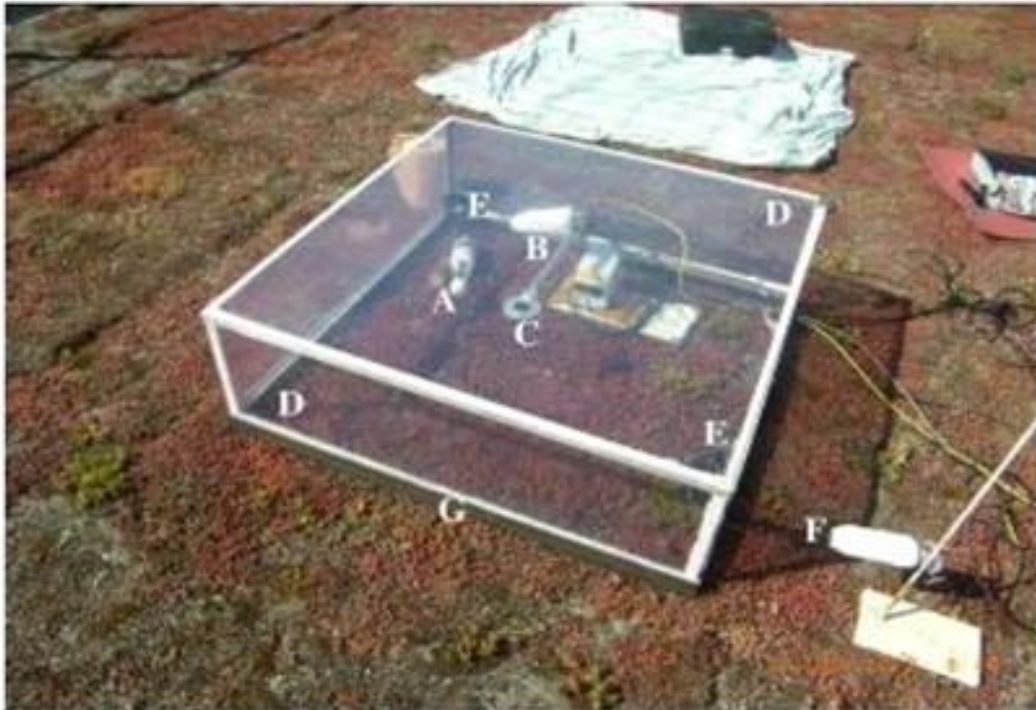
Figure S.4: Evapotranspiration chamber developed at CEREMA. The letters are defined as follows: A for Absolute humidity measure; B and F for respectively indoor and outdoor temperature sensors; C for net radiation sensor; D: PMMA enclosure and, E for the fan (Sabre et al., 2015).
